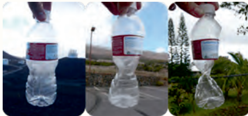
Figure 3.16 The plastic bottle (a) sealed at 4,300 m altitude, (b) the same sealed plastic bottle at an altitude of 2,700 m and (c) at the 300 m.
