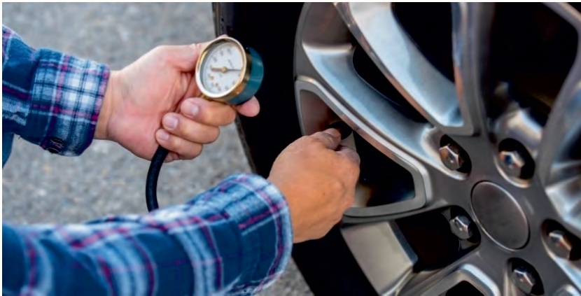
Figure 3.8 Measuring a gauge pressure of a car.
