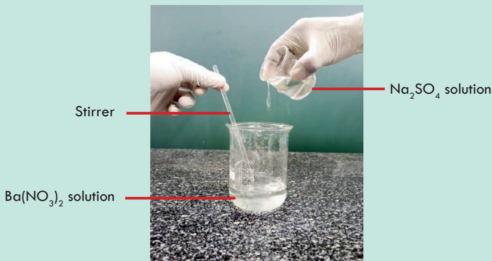
Figure 1.6 Double displacement reaction between \text{Na}_2\text{SO}_4 and \text{Ba}(\text{NO}_3)_2
