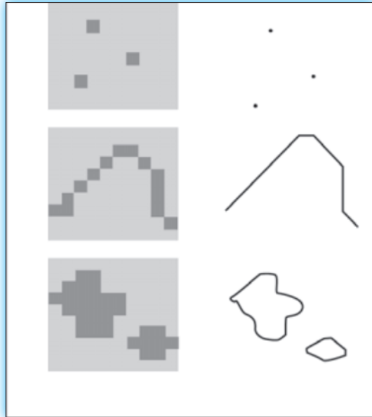
Figure 8.11: Representation of Point, Line and Area Features (Raster versus Vector)
