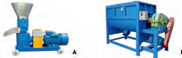
Figure 14.5. Feed processing equipment: A) feed miller, B) feed mixer
