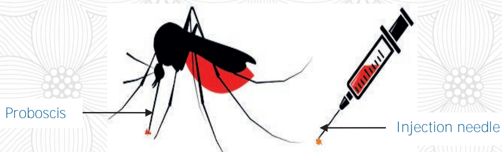
Figure 1.3 Injection needle imitated from a mosquito's proboscis
