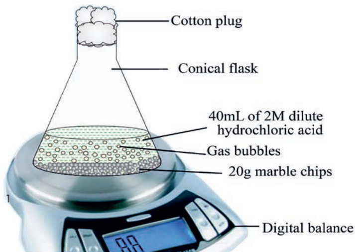
Figure 4.4: The laboratory set up for the measurement of rate of reaction
