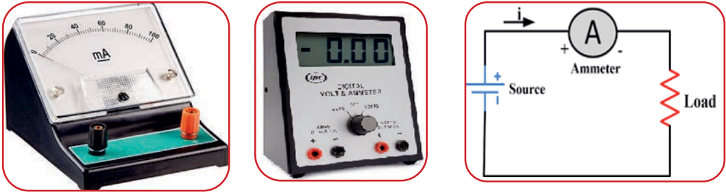
Figure 6.27: Ammeters and How to connect them.
