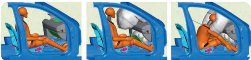
Figure 4.7 Airbag systems in vehicles are designed to deploy during vehicle collision
