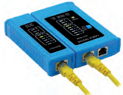
Figure 5.24: UTP cable tester
