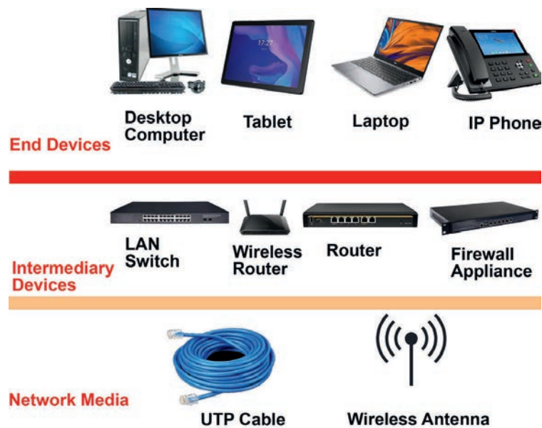
Figure 2.2 End devices, intermediary devices and media
