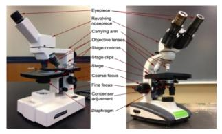
Figure 1.10 Microscope and its parts
