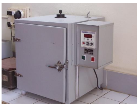
Figure 1.6. A Bacteriological incubator
