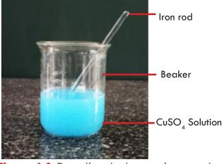
Figure 1.3 Reaction between iron and copper (II)
