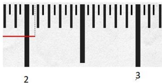
Figure 2.5: Red line and number of divisions for a given span
