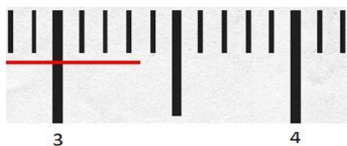
Figure 2.2: Reading the measured value of a red line
