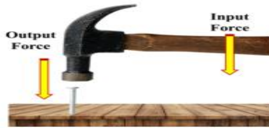
Figure 1.7: Schematic diagram of speed multipliers
